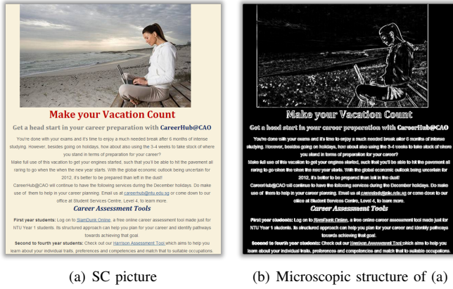
Fig. 4: Illustration of microscopic structures of screen content pictures: (a) is a pristine screen content picture; (b) is the map of microscopic structures of (a).
