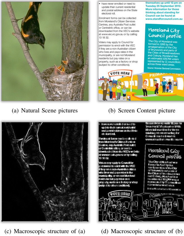
Fig. 2: Comparisons of the macroscopic structures of the natural scene and screen content pictures. (a) and (b) are pristine natural scene and screen content pictures; (c) and (d) are the maps of macroscopic structures of (a) and (b).
